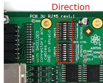
**Figure 4: Position of switches**
