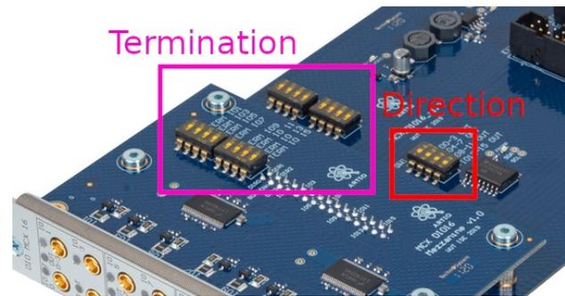
Figure 3: Position of switches
