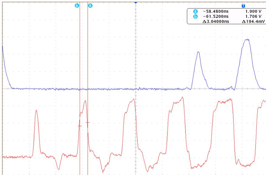
Figure 4: Minimum pulse width required for BNC-TTL card
